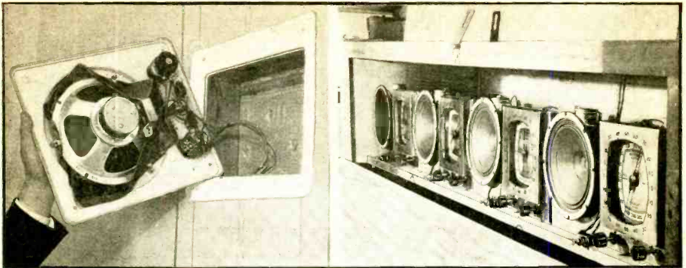
Each wall panel is easily installed and easily serviced. Here we see a rear view of a wall unit showing all components compactly and conveniently mounted on a single panel. At right is the array of 4 broadcast receivers located in an ordinary home-built box situated in the cellar of the home. Each set has its own speaker (used only for tuning-in and pre-setting of stations) and its individual master switch. (All photos—Talbran)
