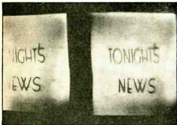
Fig. 2. Effect due to line time base operating at \frac{1}{2} correct frequency.
